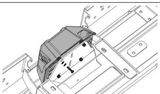
3. Attach the winch control box to the flat surface inside the bar as shown.
