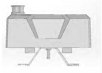
2. Secure plastic back onto control box, taking care to leave the two supplied bolts in position.
