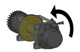
Warn / Magnum / Smittybilt winches: Undo the screws in the gearbox end of the winch. Carefully slide the gearbox away from the winch only until it is able to rotate. Rotate the gear box anti-clockwise 72° and replace screws.
