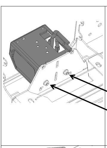
**Bushranger winches.** First remove one plastic end from the control box. Slide in two Hex head M8x20 bolts. (not provided).
