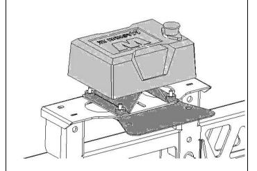
3. Attach bracket and cable protector as shown using and M6x25 hex bolts, spring washers, flat washers and flange nuts provided. Ensure the cut-out edge of bracket faces the front of the bar..
